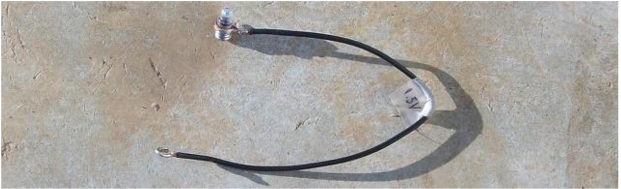
A piece of wire and a flashlight bulb are all you need to make a battery tester. The one shown above uses a flashlight bulb from a flashlight with one 1.5-volt battery. The piece of tape on the wire says "1.5 volt."
